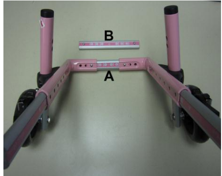
Short width connector (A) installed – wheelchair at its widest position. If your pet is wider than 6.5", remove connector (A) and insert connector (B)
